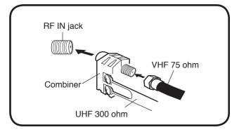
Connect the VHF 75 ohm cable and UHF 300 ohm Twin-lead Wire to the Combiner. Attach the Combiner to the RF IN Jack.
